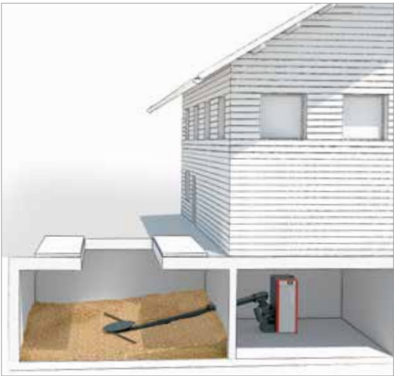
Filling of storage room via ceiling opening, transport to boiler via auger
