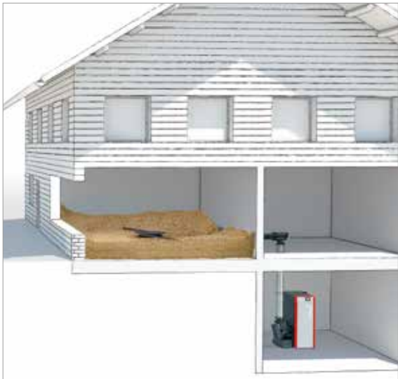
Direct filling of storage room, link to boiler via down pipe
