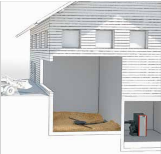
Horizontal room clearing to the boiler
