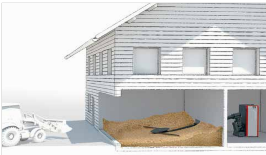
Direct filling of storage room, transport to boiler via auger
