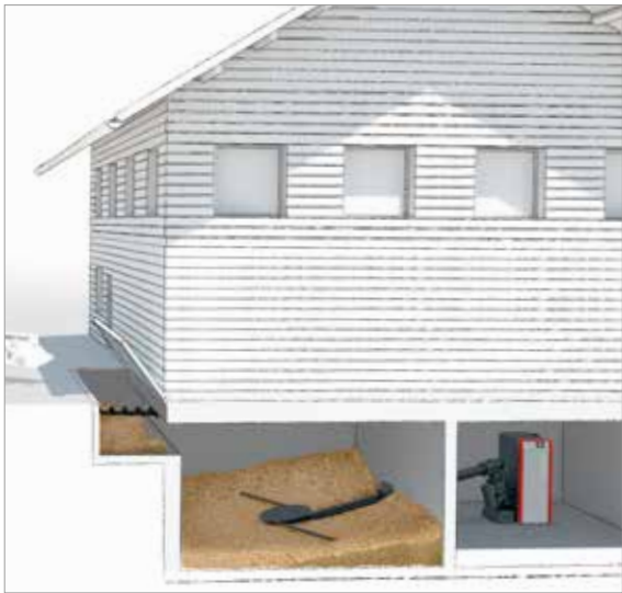
Filling of storage room via ceiling-mounted filling auger, transport to boiler via auger
